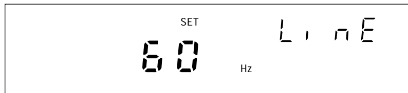
Line frequency display for setting the line frequency to 60 Hz
