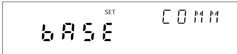
Communications display for setting the BCN
